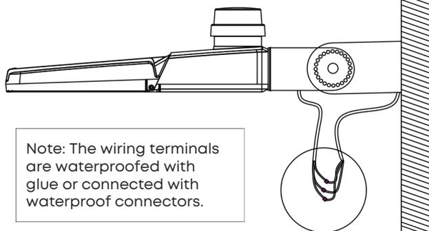
Note: The wiring terminals are waterproofed with glue or connected with waterproof connectors.
