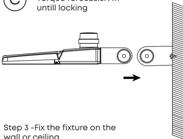
Step 3 - Fix the fixture on the wall or ceiling
