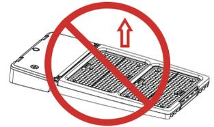
**Note:** please ensure that the lens is not mounted facing the sky to prevent water from entering the lens area.
