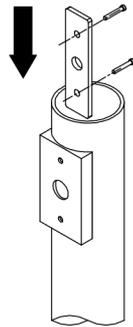
Step 1-Install the backplane and bracket adapter on the pole with top bolts, nuts and washers
