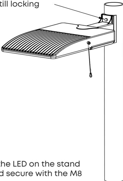
Step 3 - Fix the LED on the stand adapter and secure with the M8 screw
