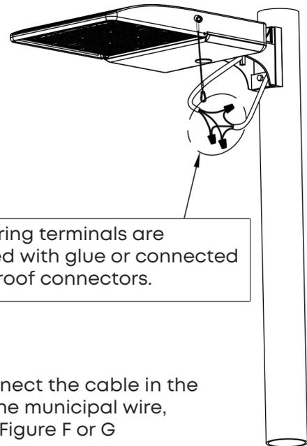
Note: The wiring terminals are waterproofed with glue or connected with waterproof connectors.
