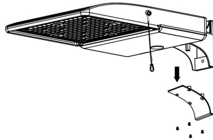
Step 2 - Remove the screw and open the cover
